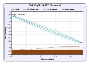
Properties Eagle Tower Bld LC1 **Height above Sea** 119 m 77 m 50 m **Antenna Height** 6 m 5.4 GHz ETSI 5.4 GHz ETSI Regulation Product ID RW5000/HBS/5200/F54/ETSI/EXT RW5000/HSU/5510/F54/ETSI/EMB RW-9061-5004 Embedded Antenna Antenna **TX Power** 17 dBm 12 dBm EIRP 30 dBm 30 dBm -75.8 dBm -70.8 dBm RSSI Fade Margin 7.2 dB 9.2 dB 0° 94.6° Azimuth -3.7° 5.2° Elevation HSS HSC INU
